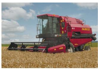
The combine harvester KZS-5 is intended for direct and windrow harvesting of cereals, it can also be used for harvesting of leguminous and rape on plain fields with slope level up to 8° using special equipment.
