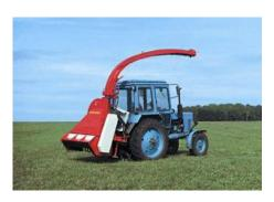
Mounted mower-shredder is intended for harvesting grass, maize and other ensilage crops up to 1,2 m high with chopping and loading into the transporter-wagons.
