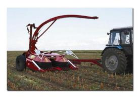
Pull-type harvester KDP-3000 "PALESSE FT40" is intended for harvesting maize, including wax-ripened and complete ripeness maize, sorgo, sunflower and other tall-stalked crops, mowing green crops, picking-up mass from swaths of prewilted sowed and natural grass with simultaneous crushing and loading into the transporter-wagon.
