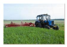
Mower-conditioner KPP-4,2 "PALESSE CT42" is intended for mowing of grass with simultaneous squashing of mowed crops and putting them into swath to the stubble. Also it can be used for grass mowing without squashing with gathering of mowed mass into swath. Operates with 1,4 drawbar category tractors.
