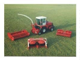
Forage harvesting complex "K-G-6 PALESSE" is intended for harvesting of maize, including wax and full-ripened maize, other high-stemmed crops, also for mowing green and picking-up slightly dried, sowed and natural grass from swaths, chopping and transporter-wagons. loading into Forage harvesting complex PALESSE" "K-G-6 includes universal power vehicle, chopping
