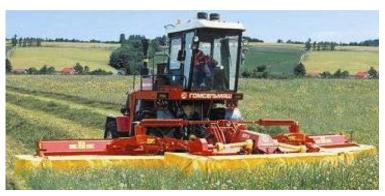
KPR-9 "PALESSE CH90" mower is intended for cutting of green seeded and natural grass with simultaneous flattering and laying of mowed mass into three swaths in conditions of temperate zone at flatland with 80 grades, with stones, which overhangs up to 40 mm above the earth surface.
