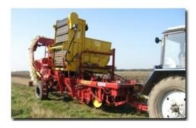
Semi-coupled potato harvesting combine PKK-2-05 "PALESSE PT25" with a bunker and a sorter desk is intended for harvesting of potato on light and mediumtextured soils in moderate climate zones of potato growing, except mountainous, with the field grade limit up to 4°.
