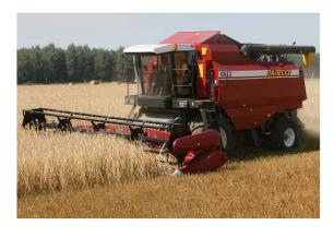
The combine harvester is intended for direct and windrow harvesting and it can also be used for harvesting of of maize, sunflowers, leguminous, cereal crops, grass and rape seeds using special equipment.
