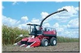
KSK-600 "PALESSE FS60" is intended for mowing down maize of any ripeness stage, sunflower and other high-stemmed crops, mowing down grass and picking up slightly dried seeded and natural grass from swaths with simultaneous chopping and loading of the mass into transport trailer.
